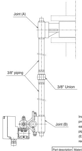
This outline dimension is for the liquid measurement. An indicator is fixed at the top of isolation valve in case of gas measurement
