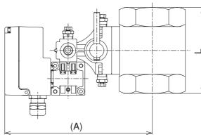
This outline dimension is for the liquid measurement. An indicator is fixed at the top of isolation valve in case of gas measurement.
