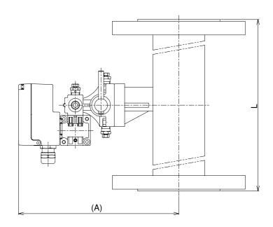
This outline dimension is for the liquid measurement. An indicator is fixed at the top of isolation valve in case of gas measurement.
