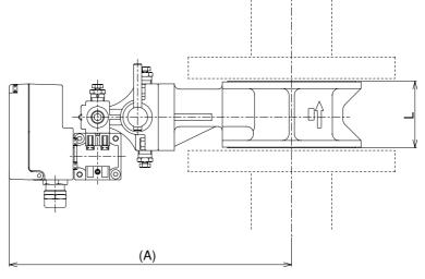
This outline dimension is for the liquid measurement. An indicator is fixed at the top pf isolation valve in case of gas measurement.
